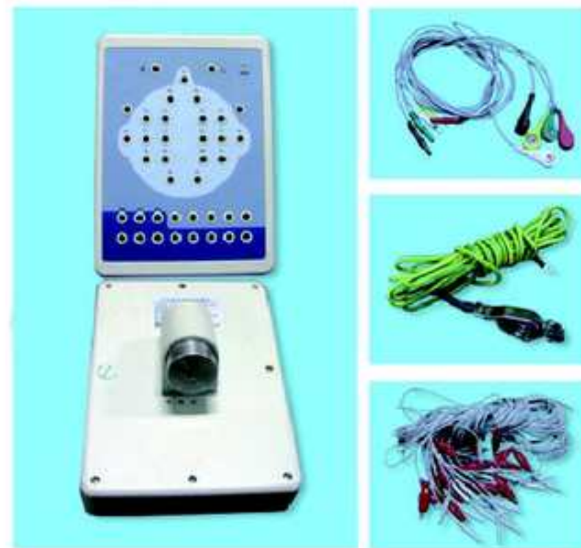
Figure (3): EEG equipment and tools. [9]
